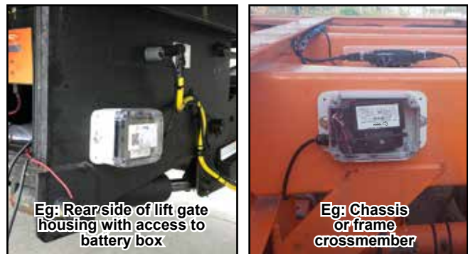
Figure 4: Suitable mounting locations (Trailer)
