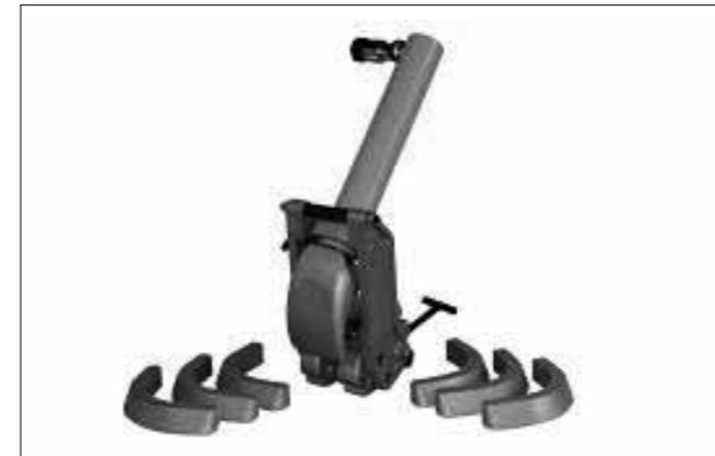
Hydraulic tire remover (tire push type) and bead wedges. Commonly used for 25 inch rims.
