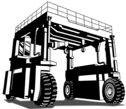
**Rubber Tired Gantry Crane(RTG)**
