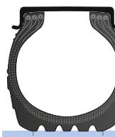
**The crown and sidewalls are formed by the same ply structure.**
