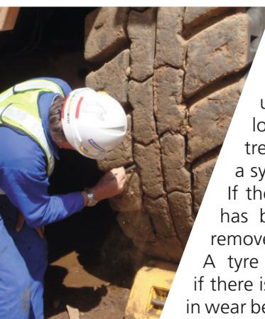
Checking for wear must always be carried out at several points on the tyre.
