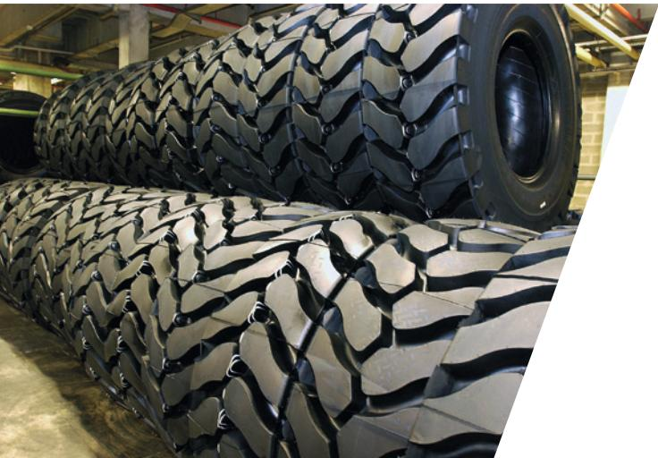
Tyres are rubber-based and are subject to natural ageing. For that storage does not adversely affect the life of the tyre, but it must be under specific conditions, limited in time, and as far as possible inside.
